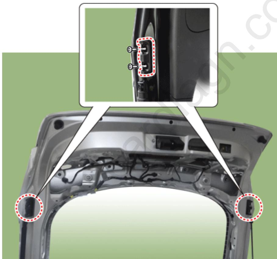
3. Loosen the rear spoiler mounting nuts.
